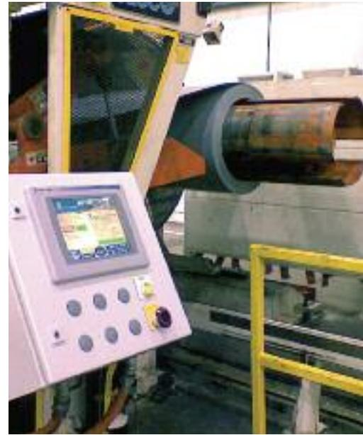
**A controls cleanup can address press-line problems caused by the addition of equipment to the line over time without planning for consistent and adequate control of that equipment. A cleanup can ease troubleshooting (with a fault log and fault descriptions easily available via the control panel or remotely), leading to increased uptime, and ease line expansion the next time around.**
